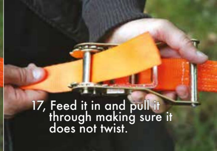
17, Feed it in and pull it through making sure it does not twist.
