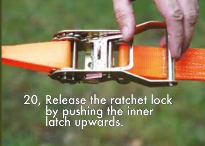
20, Release the ratchet lock by pushing the inner latch upwards.
